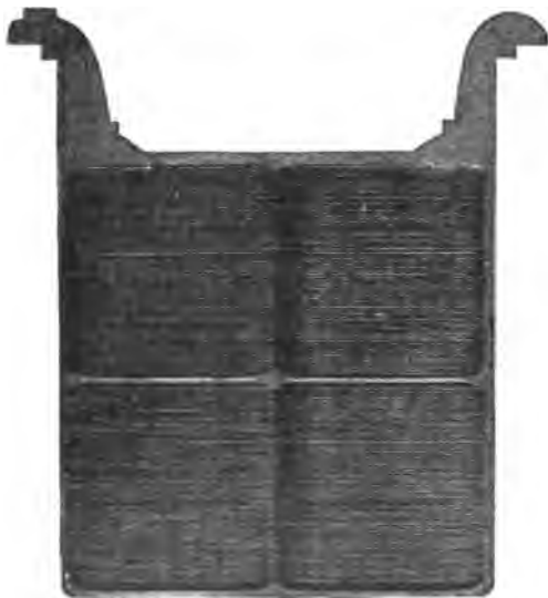
FIG. 449.—“Unformed” Plate of One Pattern of “Gould” Storage Cell. The particular plate here shown has total outside dimensions of 6 × 6 inches. The clear outline of the grooves indicates absence of oxides due to action of “forming” solutions, or charging current.
